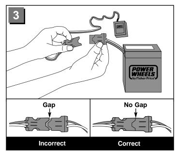
Plug the battery connector and charger connector together. Push firmly to make sure the two connectors are completely joined.
